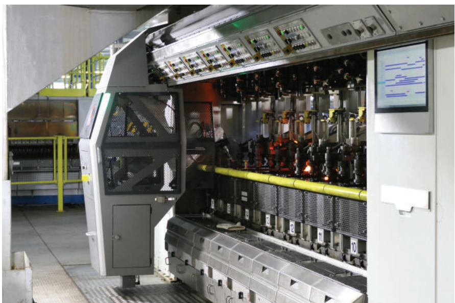
Heye SpeedLine tandem line equipped with Heye BlankSideRobot
