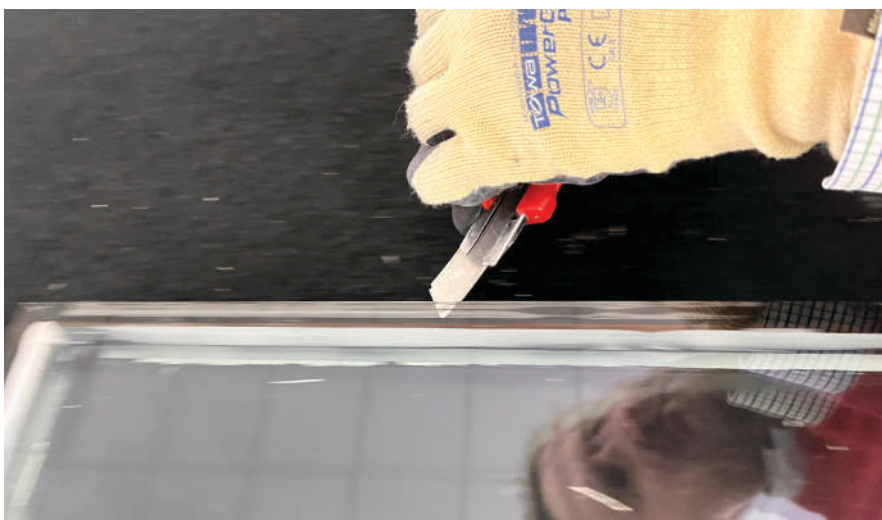
Manual separation of an insulating glass unit.
