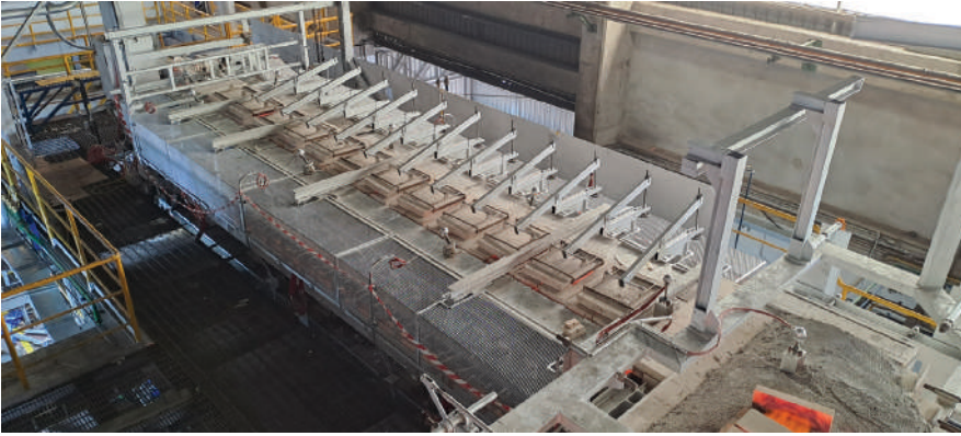
A typical Electroflex all-electric forehearth.
