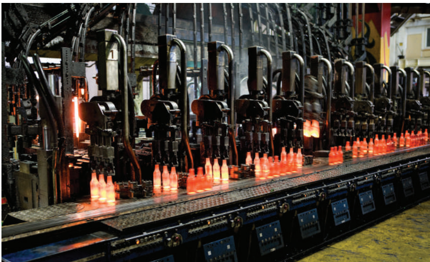
Looking at these red-hot glass bottles it is evident that glass production is highly energy-intensive. Photo: Federal Association of the Glass Industry
