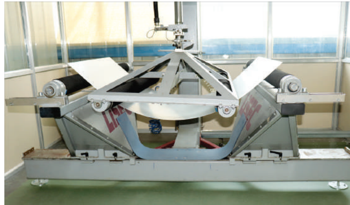
Performing a bending test on 2mm solar glass.
