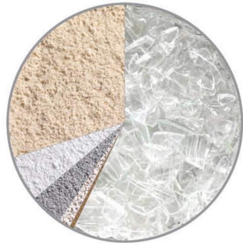
The input materials for glass production: 60% cullet, 29% sand, 5% soda, 4.5% lime, 1.5% dolomite and feldspar. Illustration: Federal Association of the Glass Industry
