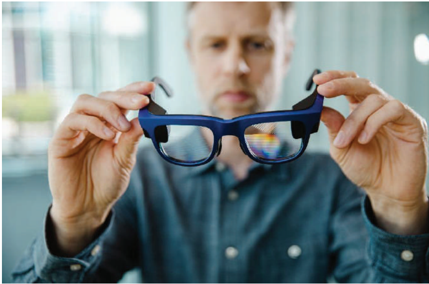
In smart glasses waveguides operate in transparent lenses to transmit digital content to the user's field of vision. Photo: SCHOTT
