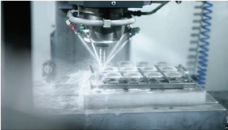
During the shaping process the (so far) square glasses receive their final shape to later perfectly fit the corresponding smart glasses. Photo: SCHOTT
