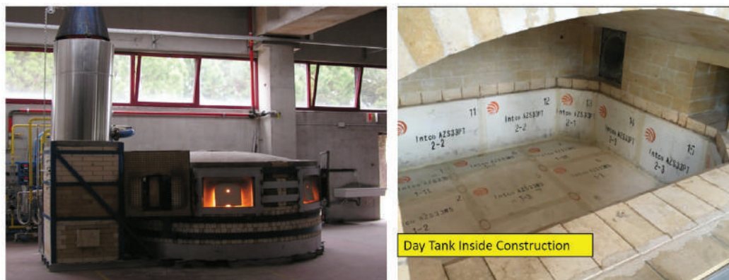
The Day-Tank Furnace is a gas fired glass melting furnace to produce soda-Lime transparent and colored glass. The range dimension is up to 4000 kg. Its main feature is the flexibility use because you can introduce raw materials subsequently melted and finally gathered.
