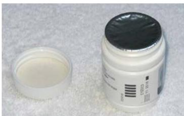
Figure 1: Example of induction sealing with screw closure and multi-layer gasket.
