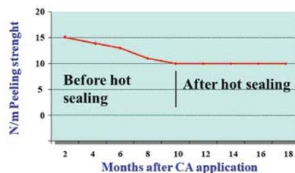
Figure 5: Typical plot of ageing to peeling performance after coupling agent (CA) glass treatment.
