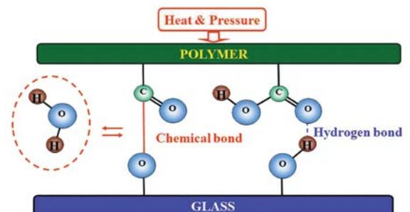
Figure 2: Simplified drawing of ionomer to glass direct sealing.
