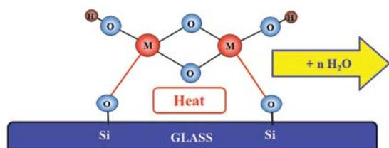
Figure 4: Simplified drawing of organometallic coupling agent treated glass.
