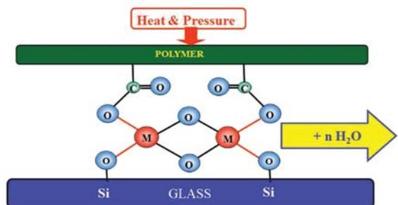
Figure 3: Simplified drawing of ionomer to organometallic coupling agent treated glass seal.
