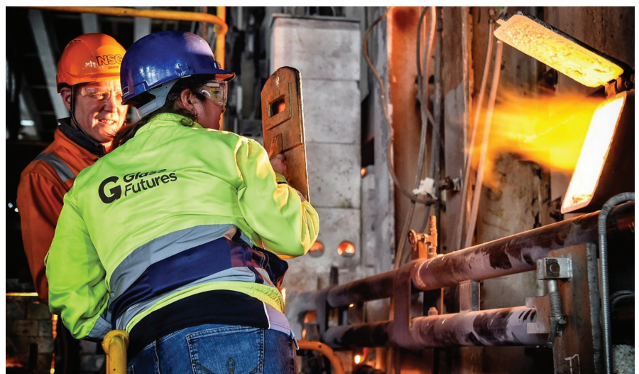
Image by Mr. Bernard Platt, taken during an industrial scale trial of biofuels at Pilkington UK (NSG Group) in 2022 that showed carbon savings of circa 70-80% of CO 2 vs. natural gas, proving
