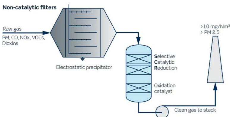
Traditional electrostatic precipitator (ESP) with tail end removal of  $\text{NO}_x$  and VOC (image: Haldor Topsoe A/S).
