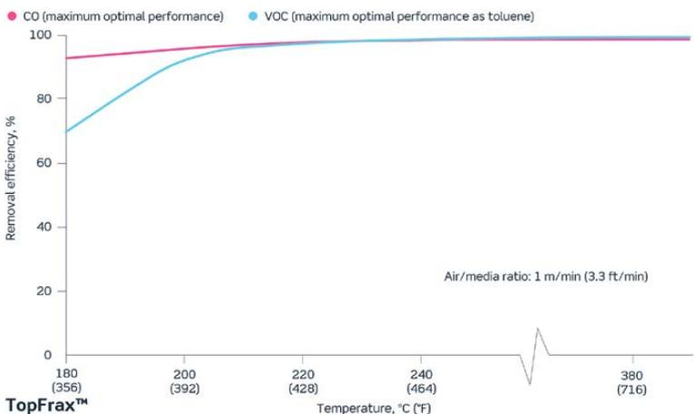
The catalytic sites on TopFrax candles oxidise CO and volatile organic compounds into harmless CO<sub>2</sub> and H<sub>2</sub>O. In addition, TopFrax OXI ensures optimal combustion of VOCs, with no additional emission of CO (image: Haldor Topsoe A/S).
