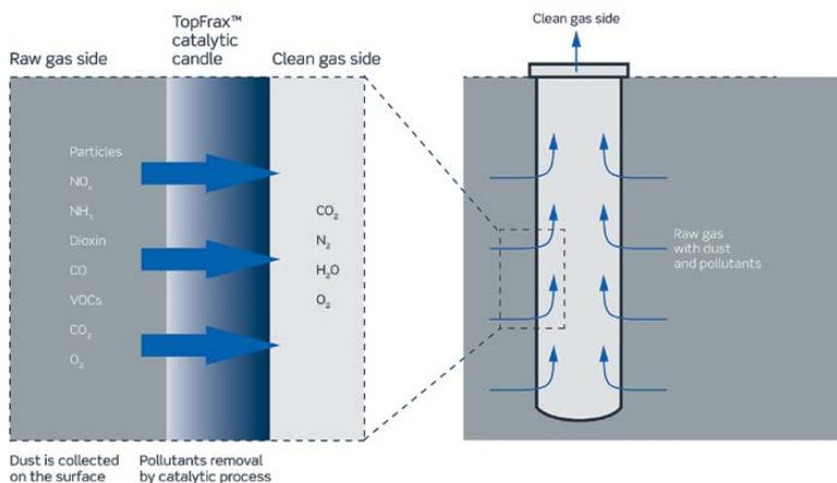
More plants are requiring a stricter emission removal system for CO and VOCs, while reducing NO<sub>x</sub> and separating the dust. Now it is possible to clean the main regulated species from practically all industrial flue gases (image: Haldor Topsoe A/S).
