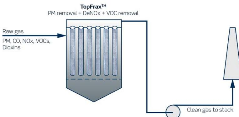
One-stage system with TopFrax catalytic filters removing dust,  $\text{NO}_x$ , CO,  $\text{NH}_3$  and VOC simultaneously (image: Haldor Topsoe A/S).
