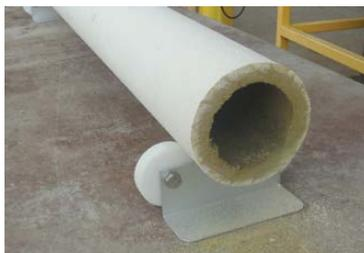
TopFrax filter cut, showing the effects of the patent-pending shell impregnation method (image: Haldor Topsoe A/S).
