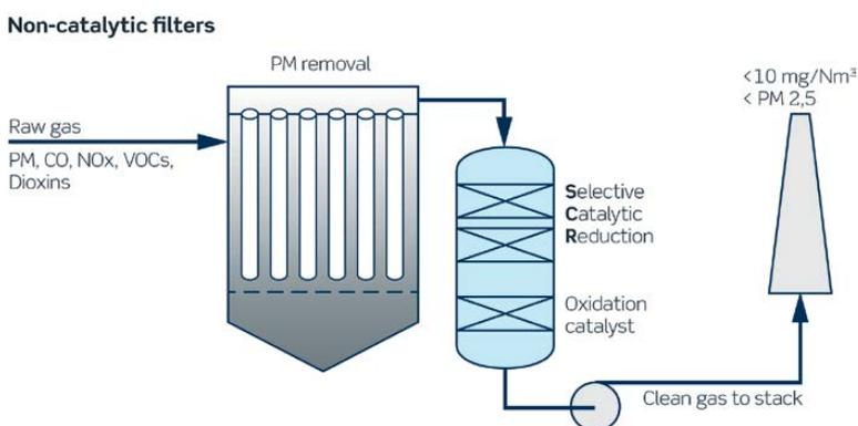
Two-stage system with initial dust removal (non-catalytic filtration), followed by tail end removal of VOC and  $\text{NO}_x$  (image: Haldor Topsoe A/S).
