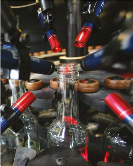
The latest Bucher Emhart Glass FLEXinspect inspection technology is installed.
