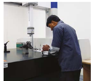
CMM inspection of parts at Accuramech's Pune facility.
