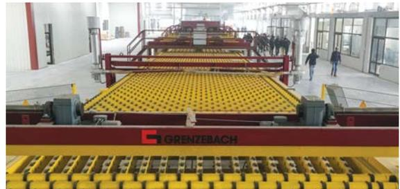
With a length of approximately 190m, the cold end equipment from Grenzebach is the end of the latest float glass production line at Gold Glass. Shown here is the main line course towards the continuous ribbon area.
