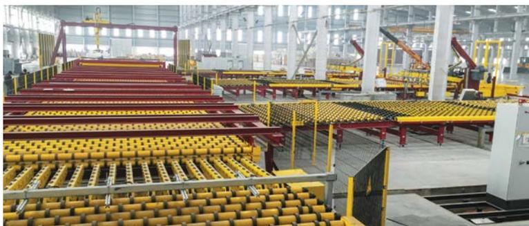
From the main line, three sidelines lead towards stackers, rotary platforms and jumbo stacker at the line end.
