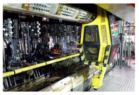
swabbing is one of the most important work steps for an IS machine operator. The robot is allowing precise and constant swabbing of the glass containers. Benefits include zero rejects from swabbing, avoidance of section stops, substantial savings on lubrication and improved operator safety.
