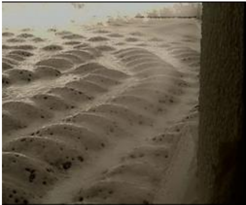
Figure 11 : glazed-over batch piles leaving the IRD doghouse
