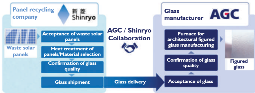
Recycling process for solar panel cover glass
