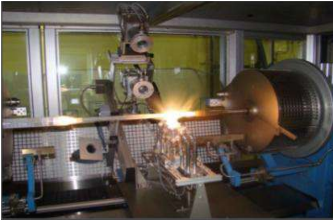
Fig. 7: MCVD-VPCD system for development of optical preform
