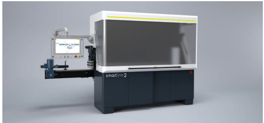
Fig. 2: SmartLine 2 Cold End inspection machine
