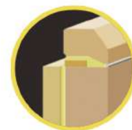
Jointing: Skewback and Breastwall
