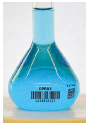
Volumetric glassware can be marked with codes linking to a product's individual certificates.
