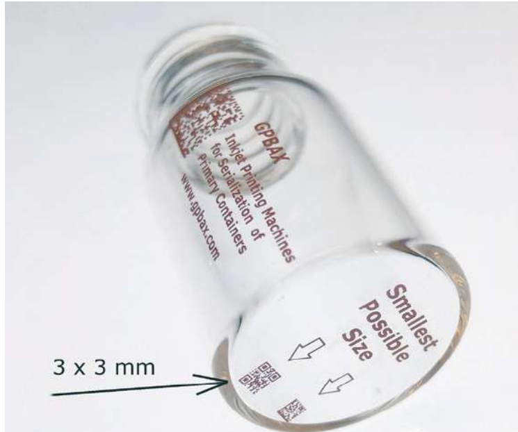
Markings applied on a small borosilicate vial (10ml), showing minimum size of traceability codes.
