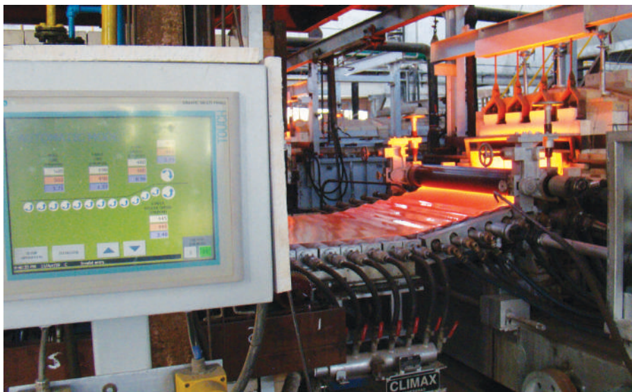
The rolled glass process at Gopal Glass Works.
