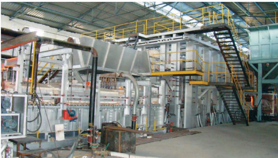
The new solar glass factory boasts a 150tpd furnace capable of producing all types of photovoltaic glass.
