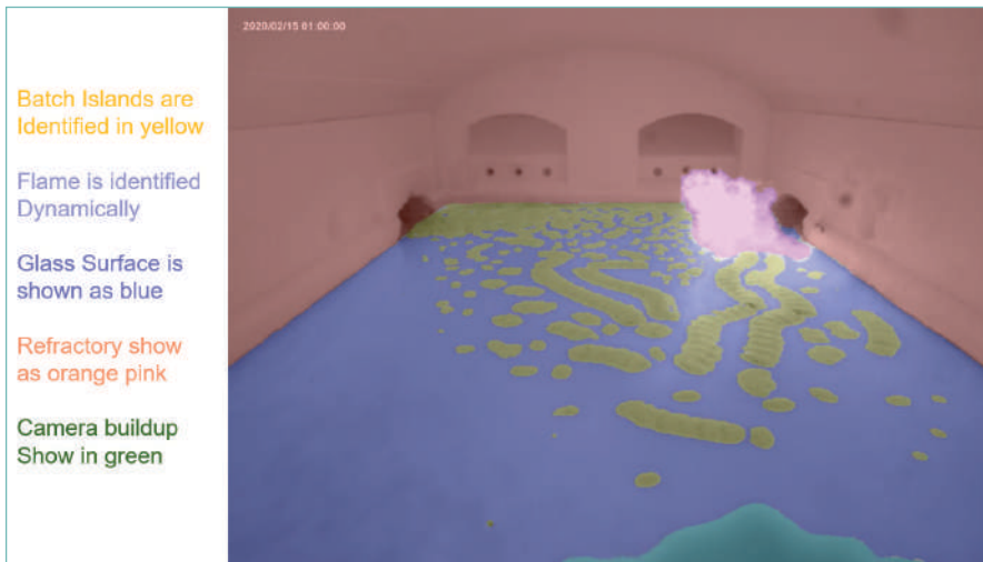
Figure 10. Furnace image from a camera identified by a Neural Network Source: Glass Service, a.s
