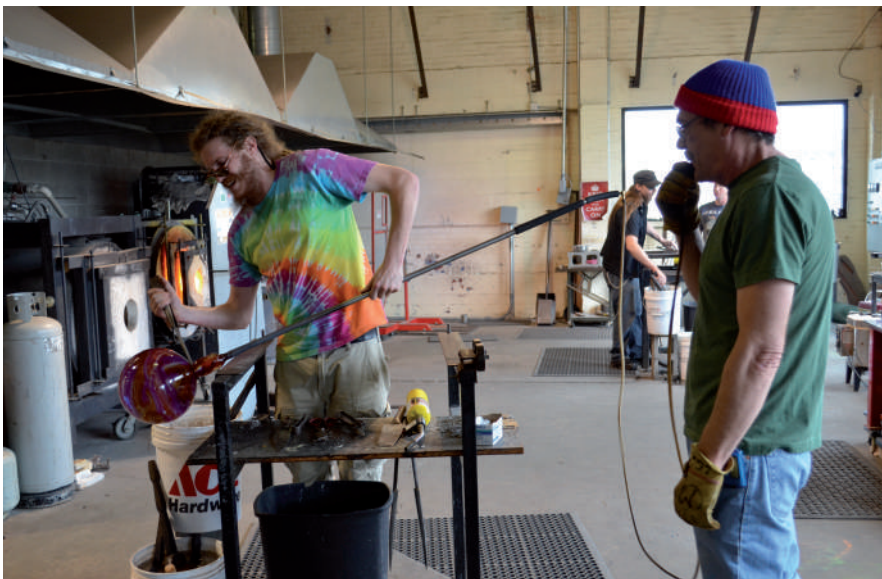
Figure 2. Glass blower at work, shaping a blown sphere before 'cracking off'.
