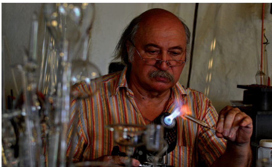
Figure 9. Lampworking, used both by the scientific and arts communities for secondary processing.
