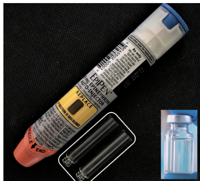
Figure 1. An EpiPen® with its Chemically toughened glass cartridges (white box); inset: a vaccine vial.
