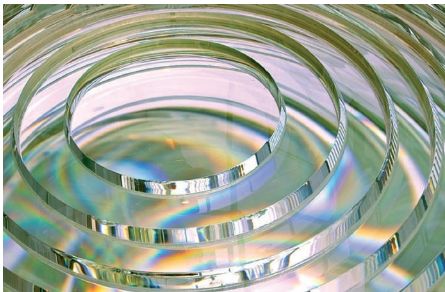
Figure 7. 3D printed optical glass artefact.
