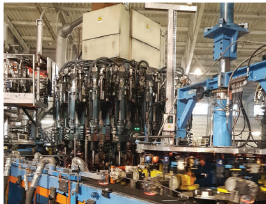
Olivotto's OGT 4.0 approach applied to a press and blow automatic forming line.
