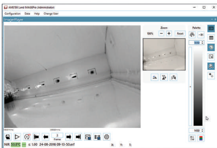
Survey mode with transportable NIR-B via an existing peephole.
