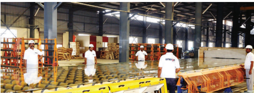
Emerge Glass produces sheet glass ranging in thickness from 1.2mm to 10mm and uses Glaverbel drawing technology to produce ultra-thin clear glass (1.2mm to 2mm).
