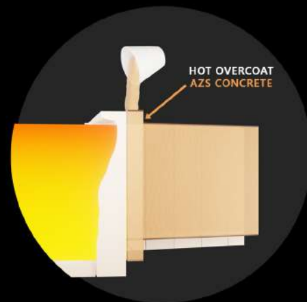
REPAIR HOT OVERCOAT AZS
