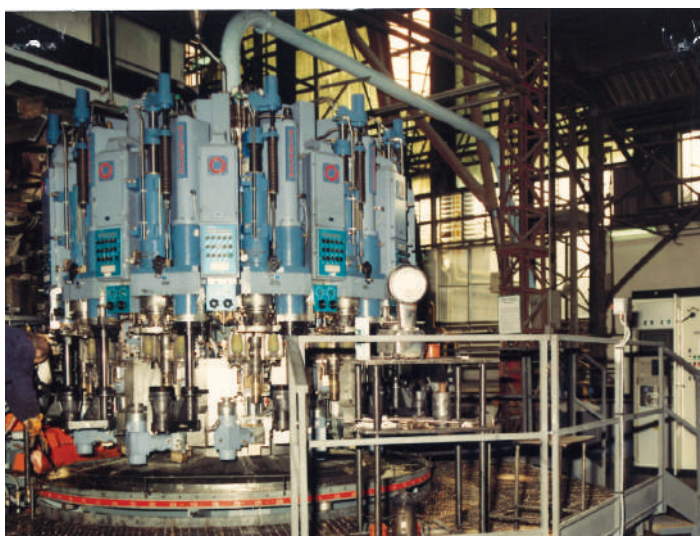
The first O.90 press and blow machine – still going strong 30 years on.
