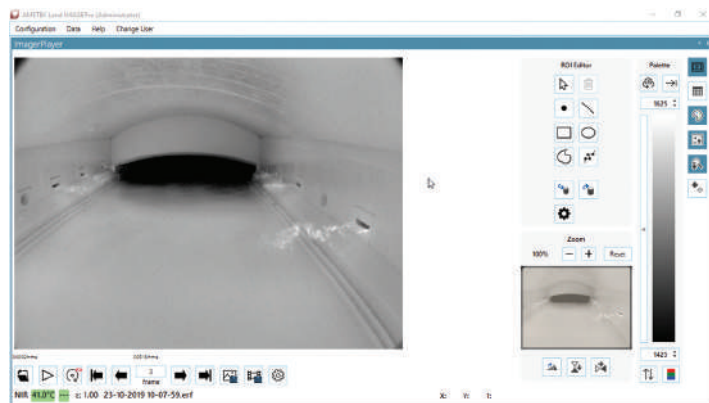
Lower temperature band 200°C greater resolution shows run-down on the L4 batch line is skewed and longer on LHS.
