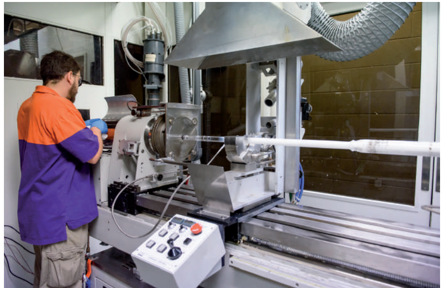
Figure 1. The deposition section of a modified chemical vapor deposition (MCVD) lathe. The white glass is the porous silica soot deposited inside of a pure silica substrate tube prior to sintering and consolidation
