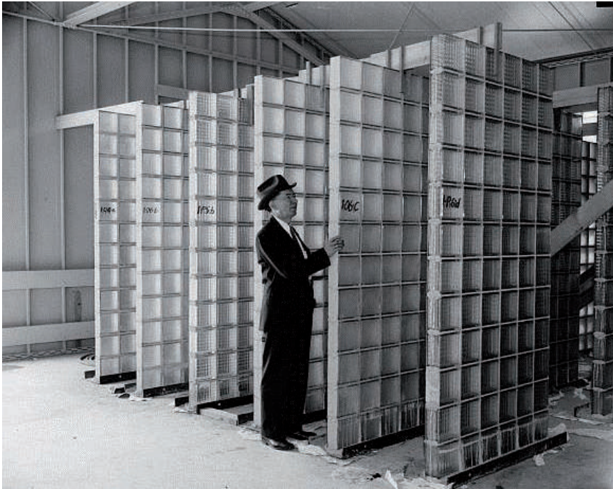
Figure 4. Bureau of Standards making extensive tests of glass building blocks (Washington DC)
