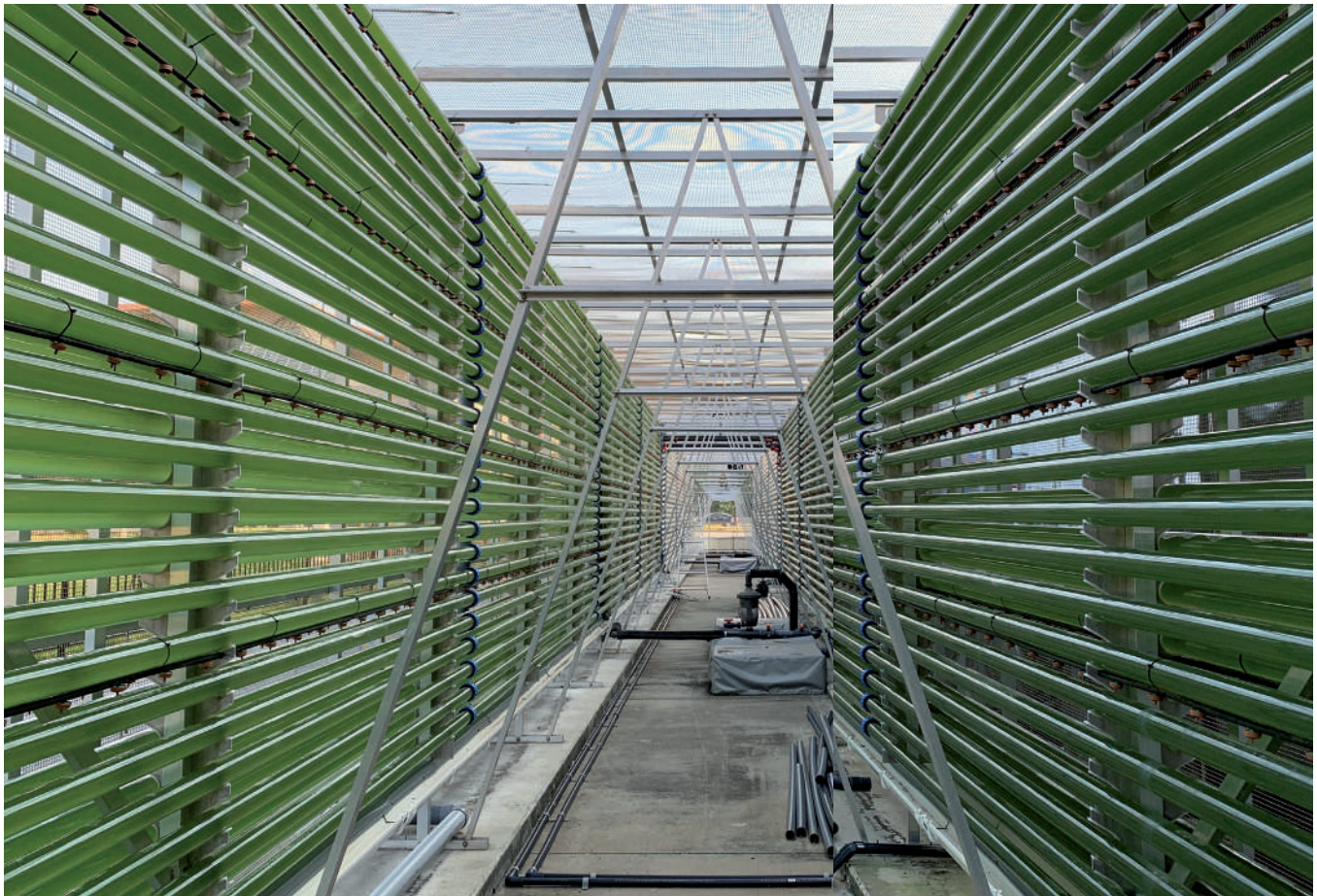
Figure 8. A photobioreactor made by Varicon Aqua for microalgae production; tubes are made of borosilicate glass
