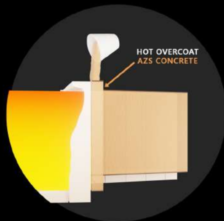
REPAIR HOT OVERCOAT AZS
