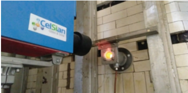
Figure 3: CO+ laser sensor for controlling the combustion process of gas mixtures.
