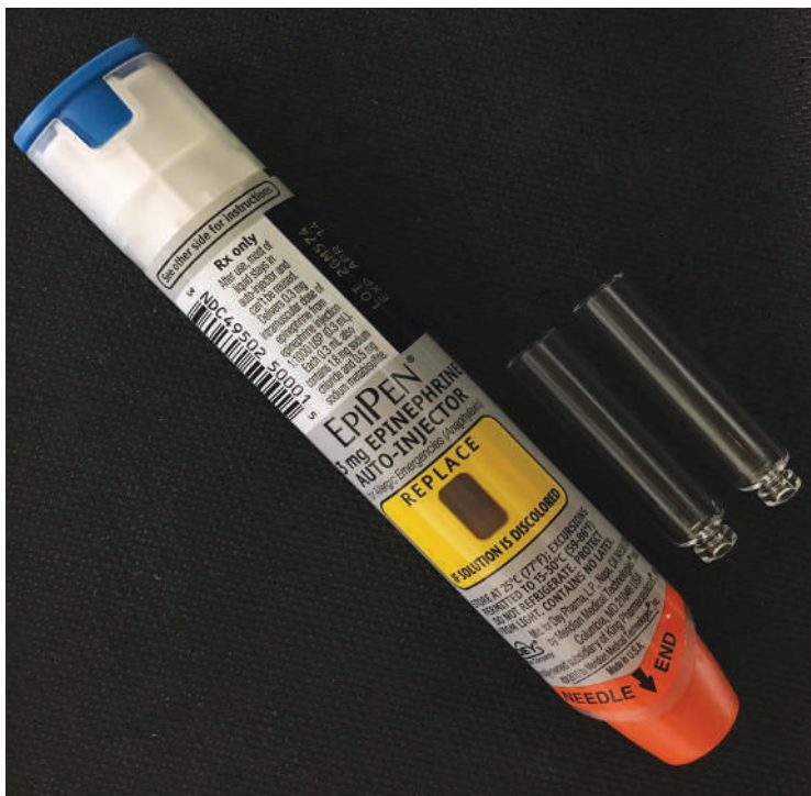
EpiPen with a Type I sodium borosilicate glass cartridge.
