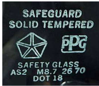
Figure-1: Safety approval markings on an automobile vent window made for a Chrysler car by PPG.
