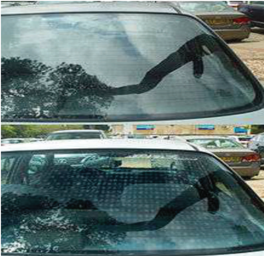
Figure 1: Tempered glass of a car rear window. Variations in glass stress are clearly seen when photographed through a polarizing filter (lower picture)
