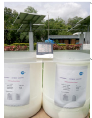
Fig: 7. Photo showing leachate test set up
