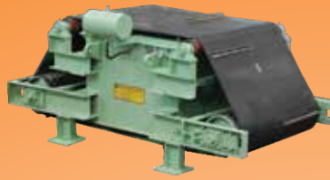
Over Band Magnetic Separator - (Operating Height From 50mm to 1000mm)
