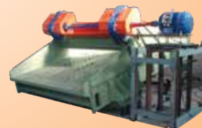
Exciter Driven Linear Motion Screen (Capacity 50TPH to 1500TPH)
