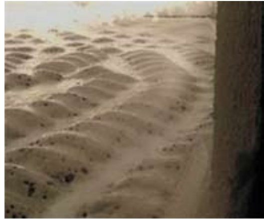
Figure 11 : glazed-over batch piles leaving the IRD doghouse
