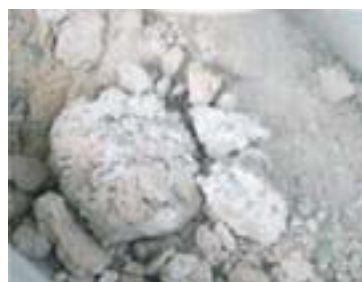
Figure 4 : typical batch clumping
