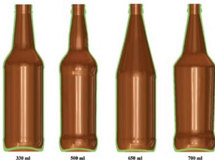
Figure 1: 3D Solidworks model for four different bottle sizes. The green coloured region represents the thickness distribution.
