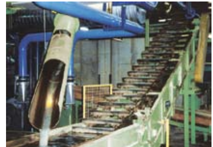
▲ (L) Five scraping conveyors working in a container glass factory operating five large furnaces. (R) Inclined discharge section of scraping conveyor.
