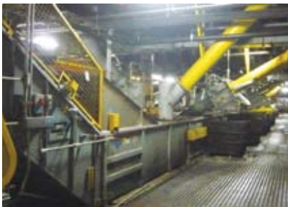
▲ (L) Five scraping conveyors working in a container glass factory operating five large furnaces. (R) Inclined discharge section of scraping conveyor.
