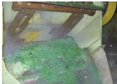
▲ (L) Five scraping conveyors working in a container glass factory operating five large furnaces. (R) Inclined discharge section of scraping conveyor.
