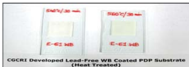
Fig. 3: CGCRI developed lead-free WB coated PDP substrate (heat-treated)
