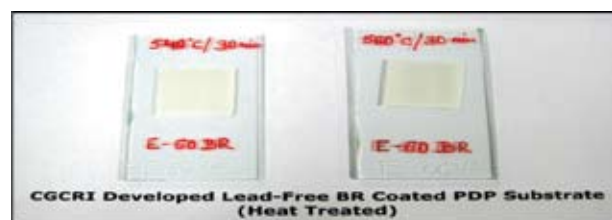
Fig. 4: CGCRI developed lead-free BR coated PDP substrate (heat-treated)
