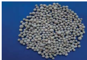
Figure 2: Specialty glass beads for nuclear waste immobilisation.
