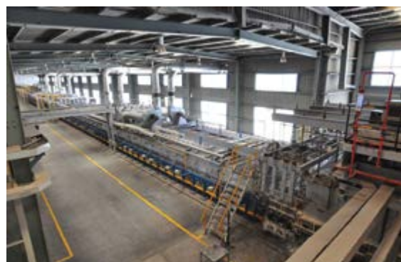
The factory features a 600 tonnes/day clear float line.
