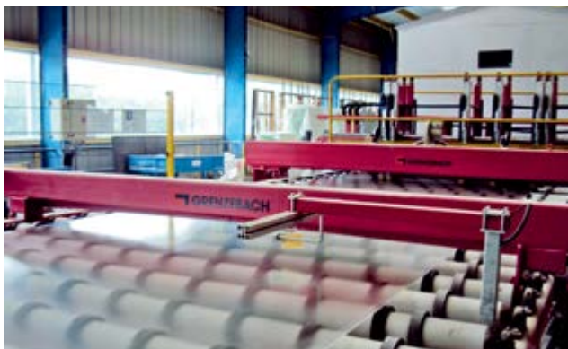
Precision cutting of solar glass at Bharuch.
